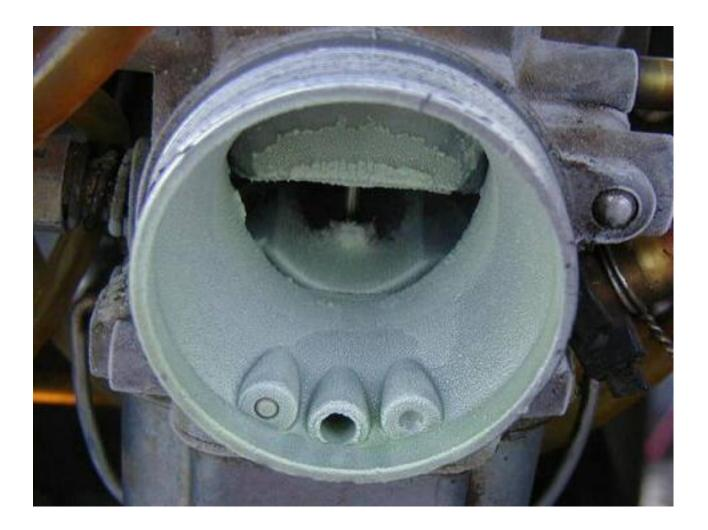
Most aeroplane engine installations attempt to prevent carb ice with an alternative hot air source, heated by the exhaust system. When applied, it will increase the temperature of the air entering the carburettor but the pilot can only guess when to apply it. Typically, when flying in suspected icing conditions, the pilot will monitor the RPM for any reduction and apply carb heat as a precaution to melt any ice before the situation becomes critical. A
